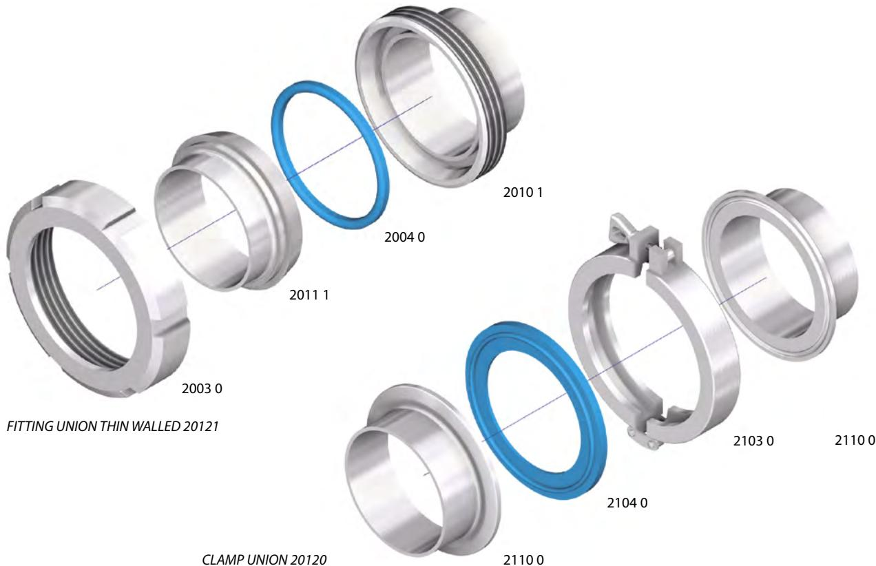
**Fitting parts** can be connected to the pipe by welding or by beading.
